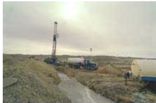
A driller empties water from a fresh well into a holding pond on a ranch near Sheridan. When the water is moved from a well, gas is released from the coal below (Kevin Moloney photo)
